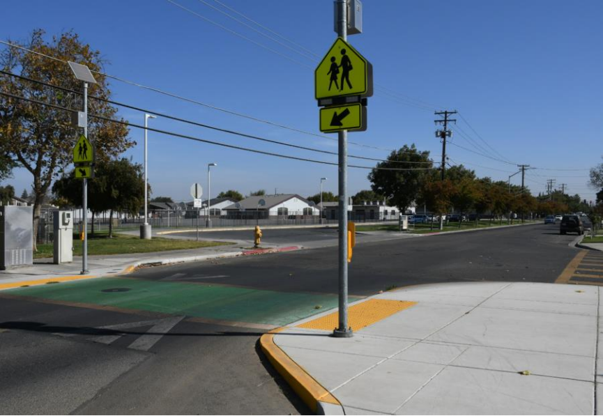
A pedestrian-activated Rectangular Rapid Flashing Beacon (RRFB) and ADA curb ramps are located near Sinclear Elementary School.
